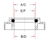
Dimension boxes H, I, L have been left blank for use in a sketch or other features that need to be added to the drawing. When measuring for dimensions E and F (o-ring touch-off) be sure that the o-ring is still installed and that the caliper blade makes only very light contact with the o-ring. Do not apply pressure to the o-ring.
