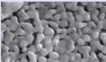
Sintered TiO<sub>2</sub> membrane (20,000x)
