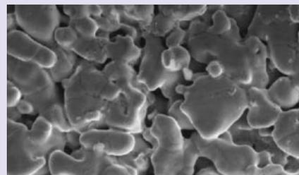
Sintered Stainless Steel membrane support (500x)
